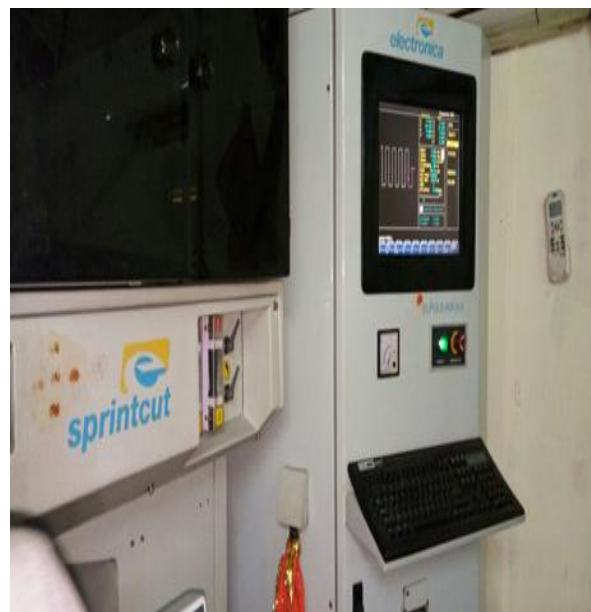
Fig 1 Control panel of EDM.
